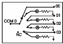
Model 1260-54 consists of six of the above 1x4 tree multiplexers. Each channel has the capability of being terminated to an optional 50Ω terminator. One tree is shown.
